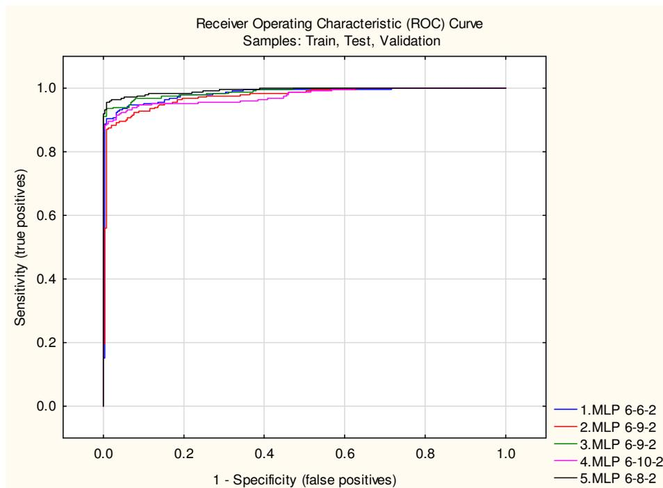
**Fig. 4.** ROC curves for different configurations of NN-DB ensemble.
